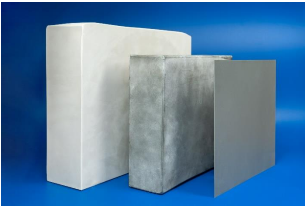
Figure 3: green and sintered \text{Si}_3\text{N}_4 blocks and multi wire cut substrate of 7.5 \times 5.5 inch and 300 \mu\text{m} thickness.
