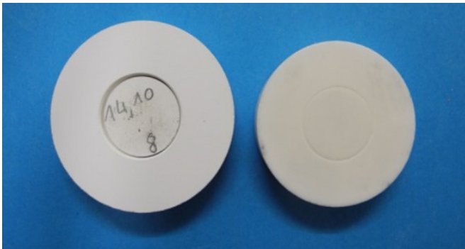
Conditioned and pre-sintered shaft and hub (left), joint state (right), Al_2O_3 .
