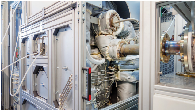
Hot gas filtration test rig for honeycomb filters or filter candles.
