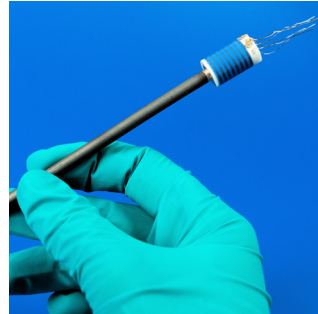
Thermocouple assembly with sensor part, reference point and electrical contacts.
