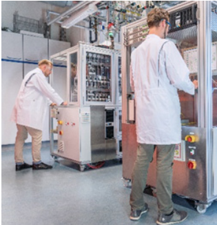
Lab-scale plant for the development of power-to-X processes.
