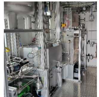
Container-based plant for the production of Fischer-Tropsch products from CO 2 and water.
