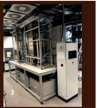
1 Membrane electrolyte system in laboratory scale.
