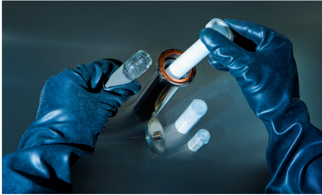
Assembling of a Na/NiCl 2 battery cell.
