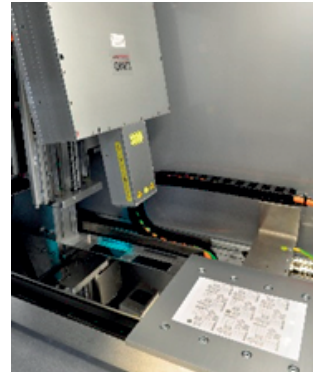
Diode laser line for millisecond processing.
